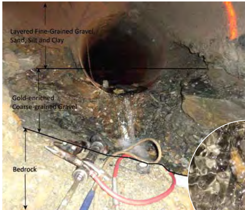
Middle (left to right): • Sluicing ore to recover gold at Wingdam • Steel pipe driven into Wingdam gravels
